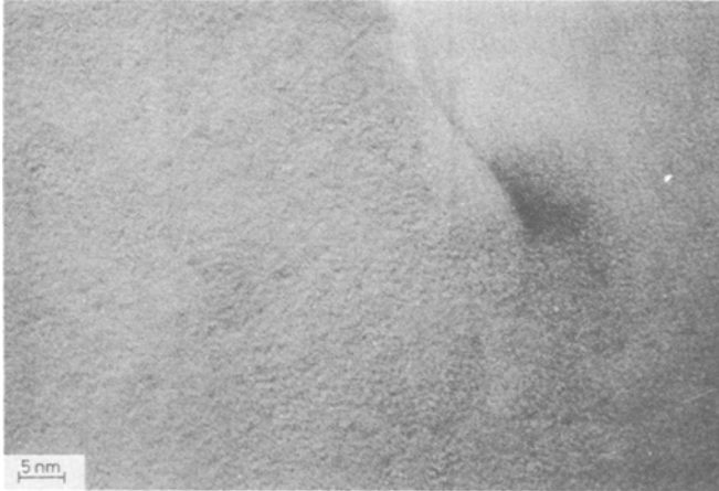
Fig. 3 High resolution image showing the (111) plane lattice fringes (taken in symmetrical position). GP-zones are visible as dark spots of irregular shape extending over several lattice fringes. A dislocation is also present, to the right of which GP-zones are absent over some distance
